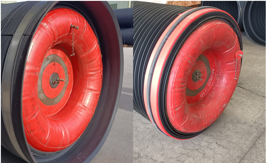
Figure 6 Picture of the inflatable stoppers sitting in the Socket (left) and Spigot (right)
