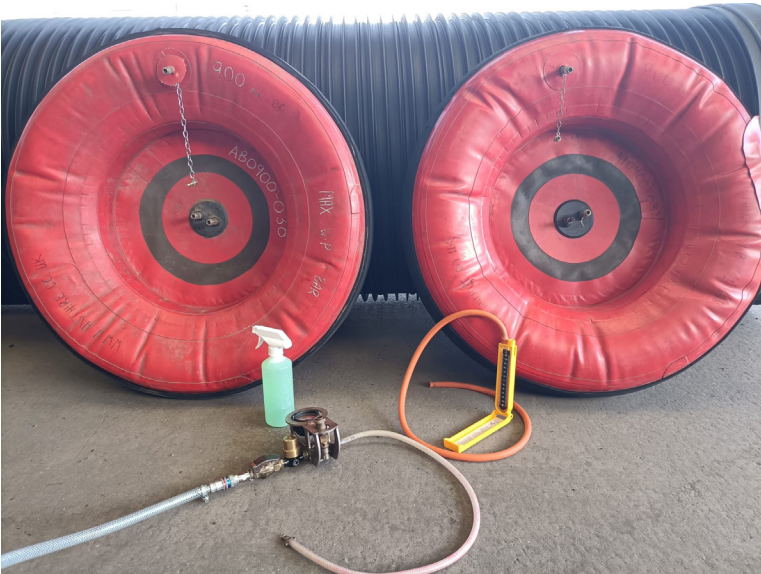
Figure 2 This picture shows two Milltest inflatable stoppers, u-gauge manometer, soapy water applicator, and airline regulator
