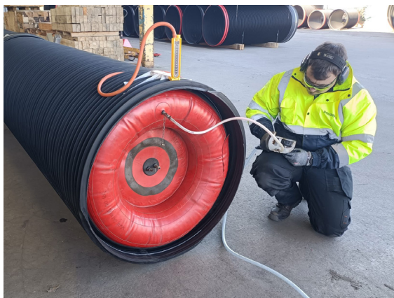
Figure 8 Picture of inflatable stopper being inflated between the marked lines in the plain ended pipe
