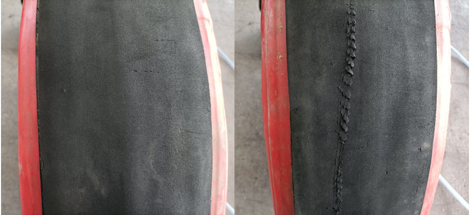
Figure 3 Picture showing the stopper surface that will be in contact with the internal surface of the CSR pipe. The picture on the left shows an undamaged stopper surface where the picture on the right shows a damaged surface
